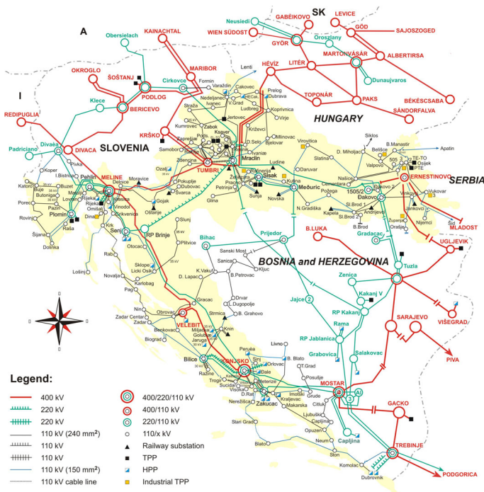
Figure 1 General network configuration of the HR system
